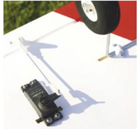
*Since each aileron has its own servo, flaperon mixing is an option.*
